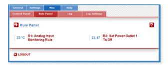
For supervision purpose, the administrator can create special accounts which display only some specific rules. In the example below, the user Bill has the possibility to supervise 2 rules and to see on a glance the rules which have been triggered.
