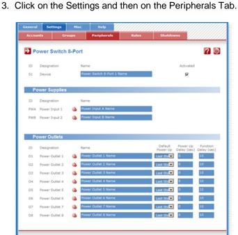
If the Power Switch is properly connected to the Power Switch Master 8-port it will be automatically recognized and displayed on this page after a delay of up to 60 seconds. In this case, the colour of the corresponding Edit and Info symbol is red.
