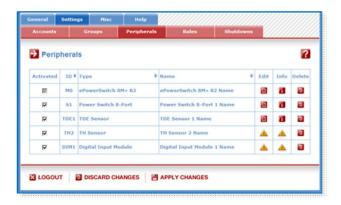
The Peripherals page is used to configure all peripherals connected to the Power Switch 558MA.
