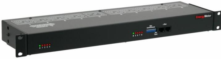
EnergyMeters can be attached to the Power Switch Master 8-port to monitor the energy consumption (kWh) and the current consumption (Amp RMS) of eight electrical devices (PC, server, light, printer...) and trigger actions if predefined limits are exceeded. The EnergyMeter is also able to monitor the Input voltage of both 16 Amps power inputs.
