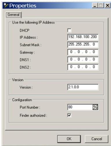
This page enables to define all IP parameters of the Power Switch Master 8-port device and displays the version of the Firmware. The HTTP protocol is enabled and the Finder program is authorized at factory settings.
