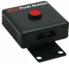
Push buttons can be attached to the Power Switch Master 8-port to trigger manually pre-programmed actions.
