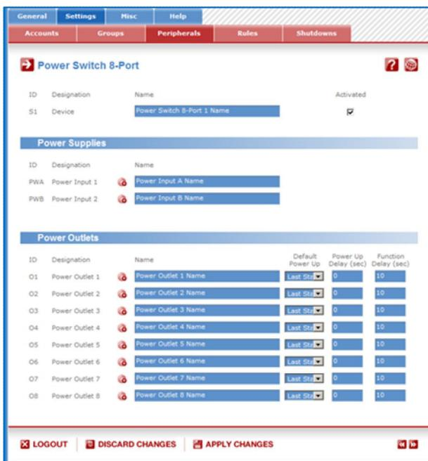
If the Power Switch is properly connected to the Power Switch Master 8-port it will be automatically recognized and displayed on this page after a delay of up to 60 seconds. In this case, the colour of the corresponding Edit and Info symbol is red.
