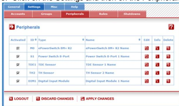
If the sensor is properly connected to the Power Switch Master 8-port it will be automatically recognized and displayed on this page after a delay of up to 60 seconds. In this case, the colour of the corresponding Edit and Info symbol is red.
