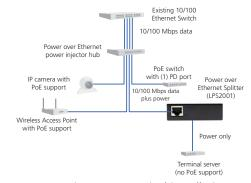
Figure 4-1. Typical installation.
