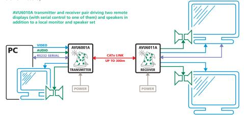
The AVU6010A transmitter and receiver modules are also available separately and are known as the AVU6001A and AV6011A respectively. Expansion is made possible by connecting further transmitters to the original AVU6001A transmitter module, however, the serial connection cannot be cascaded in this manner. Where cascades with serial connections (as well as video and audio) are required, use the AVU6004A/AVU6008A transmitters.
