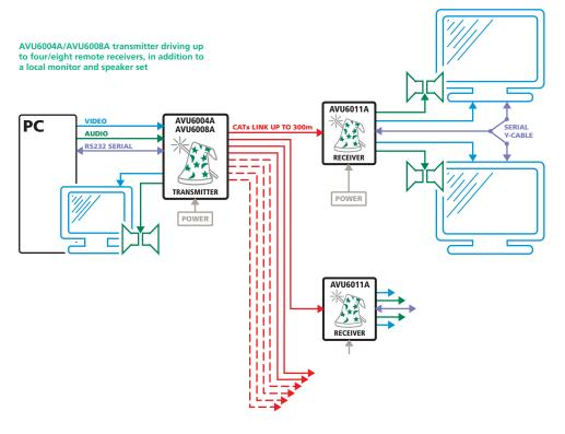
Additional expansion is also possible by connecting further transmitter modules to the original module in a cascade arrangement, each supporting their own multiple AVU6011A/ AVU6111A receiver modules - See *Expansion via cascade links* for details.
