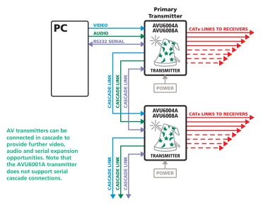
Note: The AVU6001A transmitter supports video and audio cascade connections, however, the module does not include a serial out connector and cannot support cascaded serial connections.
