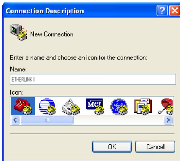
5. Then the "Connect To" window is displayed. Select the COM port connected to the subrack, minirack or SA-DESKTOP-x in the "Connect Using" drop-down menu. Click "Ok".
